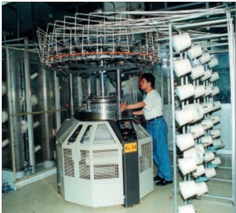
Habi-Tex, the first ISO 14001-certified company in Syria, specializes in knitting, dyeing and sewing cotton garments, mainly for export to Europe and the USA. Seen here is a circular cotton knitting machine.
